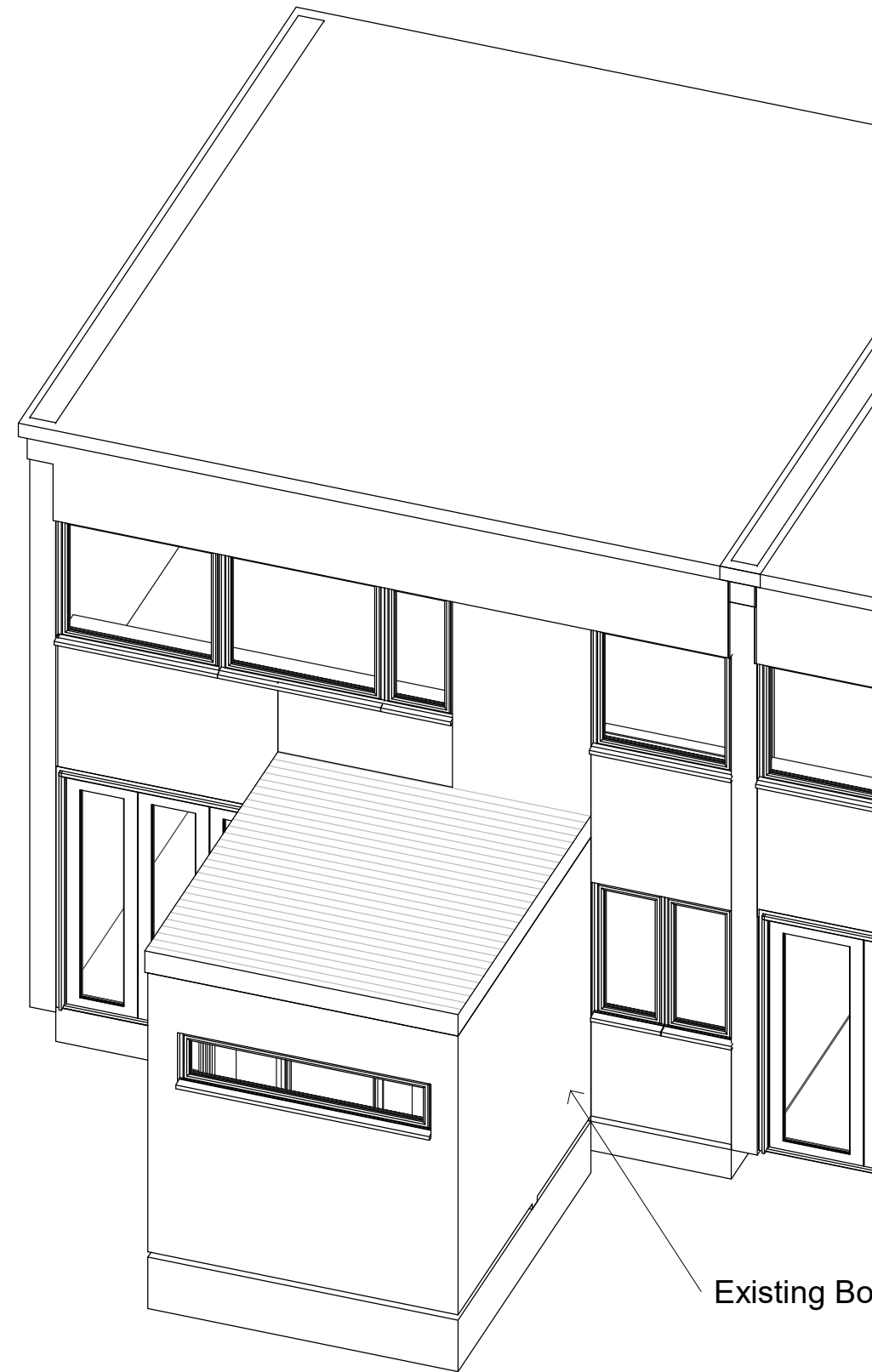
3 Volume Volume of Existing Boiler room = 3.04m3 Volume of New Shower room = 18.44m3
